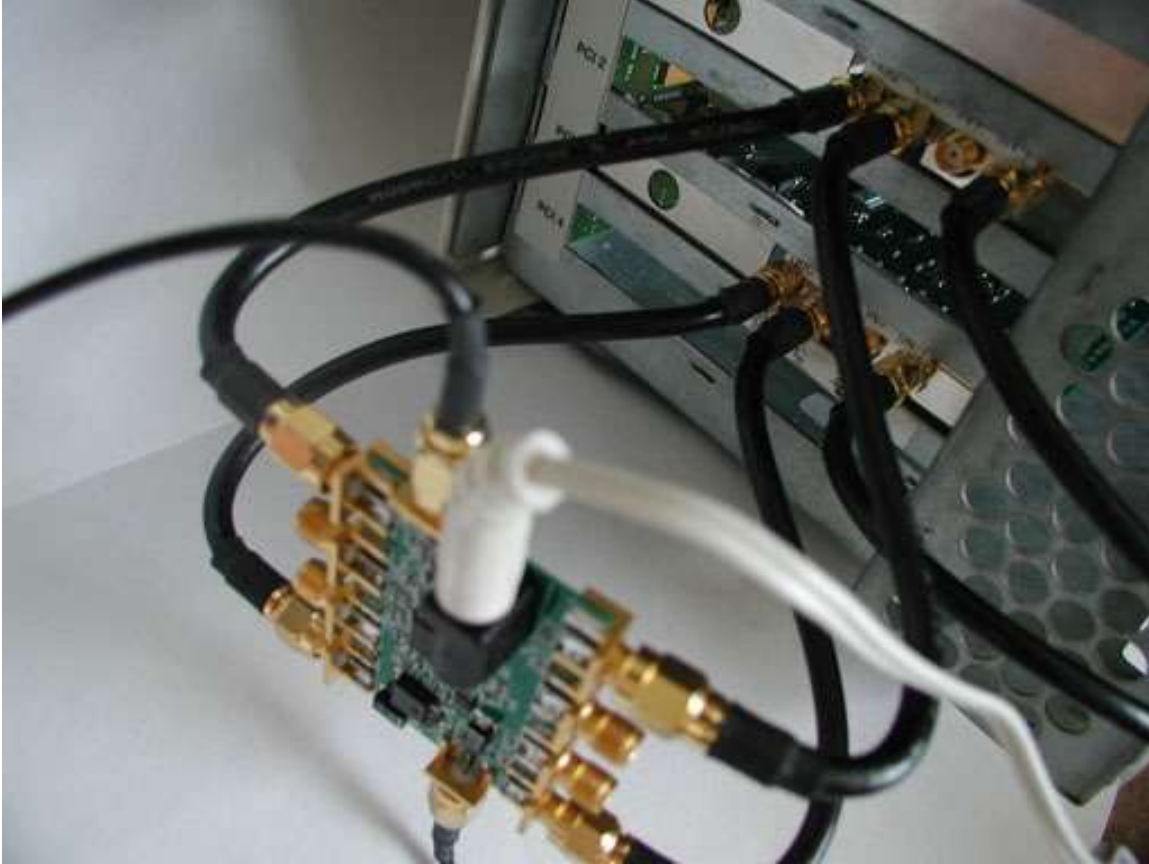
Figure 7-7.1. Connection of AD8-SPLIT2/4 to two AD8-1500DMA or DA8-1250DMA boards installed in a Sun host system. The left two thick black cables are the TRIG0 and TRIG1 outputs, and the middle two thick black cables are the CLK0 and CLK1 outputs. The black cable going into the top of the AD8-SPLIT2/4 boardlet is from the RF clock source, and the bottom black cable is from the TTL trigger source. The white cable is the +5V DC input from the included wall-cube adapter. The rightmost two thick black cables connected directly to the AD8-1500DMA boards are the signal inputs for the two boards.
